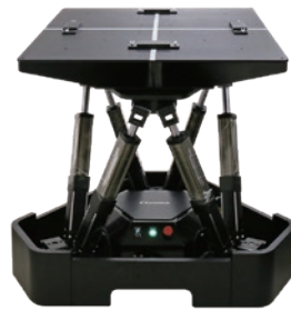
6-axis WPT test platform
