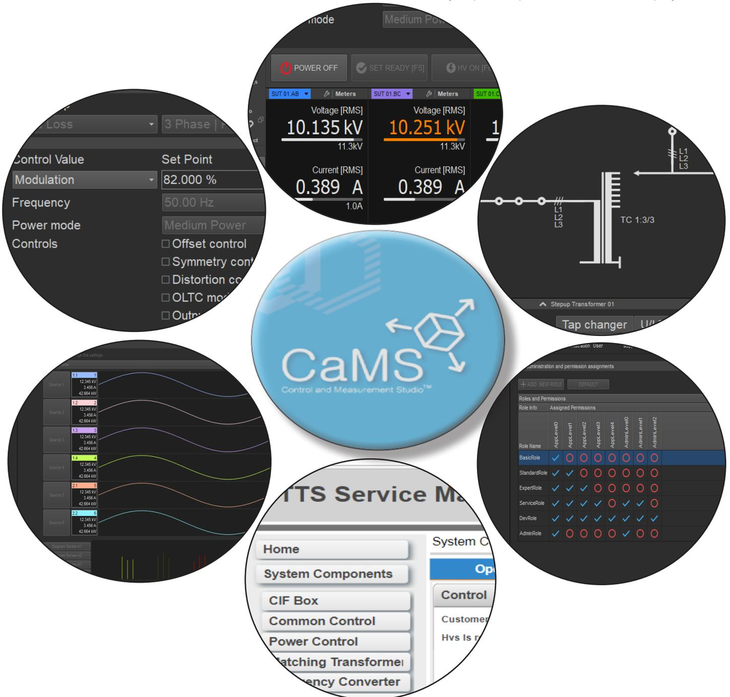
System components are simplified glyphs on the visualization pane. Specific control and status widgets are embedded in the representation. Open/closed contactors are visualized open or closed on the screen. Manual switches can be visualized as well. One single screen shows test **configuration, status** and **alarms**.
