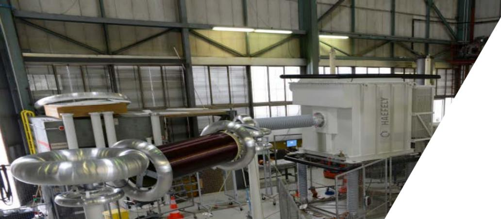
On site withstand voltage testing is an essential part of a cable laying and commissioning project. Cables and accessories are tested separately during routine testing in the factory. Testing on site is a check of proper assembly of cable and accessories together.
