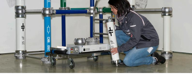
The KIT 4.0 is a high voltage system made of easily configurable elements. Due to its modular design, it is the ideal tool kit for conducting experiments in an university, in a R&D lab, or for a research application. A variety of experiments are possible with the generated AC, DC, and impulse voltages. Configurations are not only easy to put together, they occupy very little space. A fully assembled experiment occupies an area of 12 m2 and a volume of approx. 30 m3.
