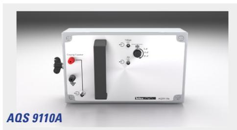
**AQS 9110a** The AQS 9110a measuring impedance is a fully passive measurement system optimized for use with the DDX 9101b as well as previous HAEFELY PD detectors. It is equipped with a user selectable three positions internal voltage divider.
