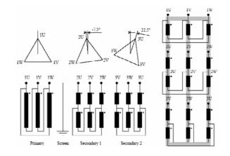
With the optional arbitrary phase shift software key (2293/ SKAP), the 2293 can measure turns and voltage ratio, phase displacement and excitation current of these special type transformers.
