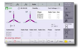
The specially developed algorithmic included in compensated mode reduces the influence of leakage flux while using low voltage, giving results much closer to the nominal ratio.
