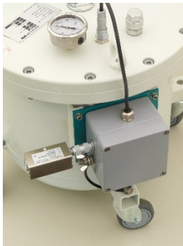
Type 3370 NK/30 standard capacitor used for connection of a 3723 resistance unit
