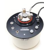
Liquid test cell for measurement of C, tan  $\delta$  and DC resistivity on liquid dielectric samples. To be used together with the measuring instrument 2830/2831:
