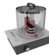
Solid test cell for measurement of C, tan  $\delta$  and DC resistivity on solid dielectric samples. To be used together with the measuring instrument 2830/2831:
