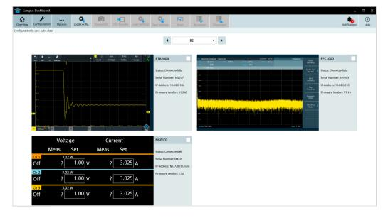
View all instruments on a bench on your computer screen using the R&S®CDS campus dashboard software; the software also supports remote control of each instrument
