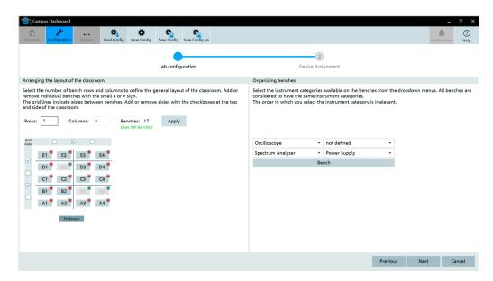
Match software layout to your lab arrangement and organize individual benches with up to four instruments
