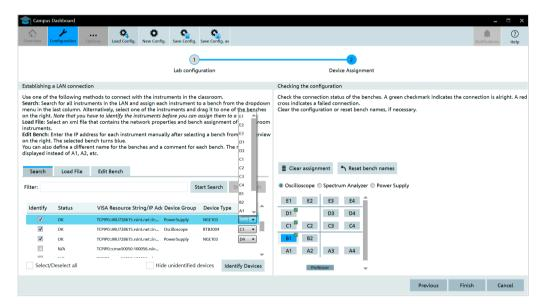
Search for supported instruments in your local network; drag & drop instruments onto individual benches
