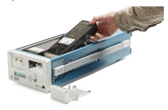
Plugging TSO8C18 module into TSO820 mainframe.
