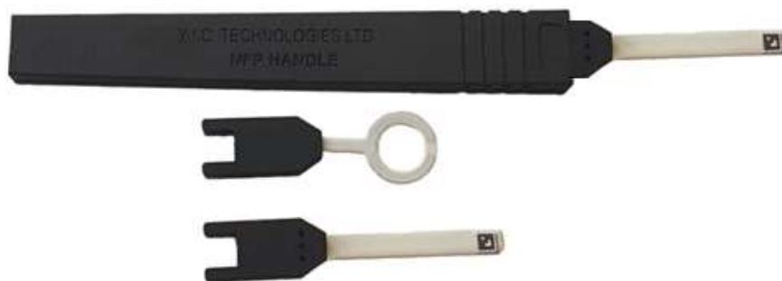
Y.I.C. Technologies set of EM probes kit designed for measuring near field radiated emissions for EMC/EMI pre-compliance testing.
