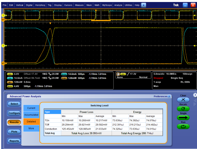
Switching Loss measurements.
