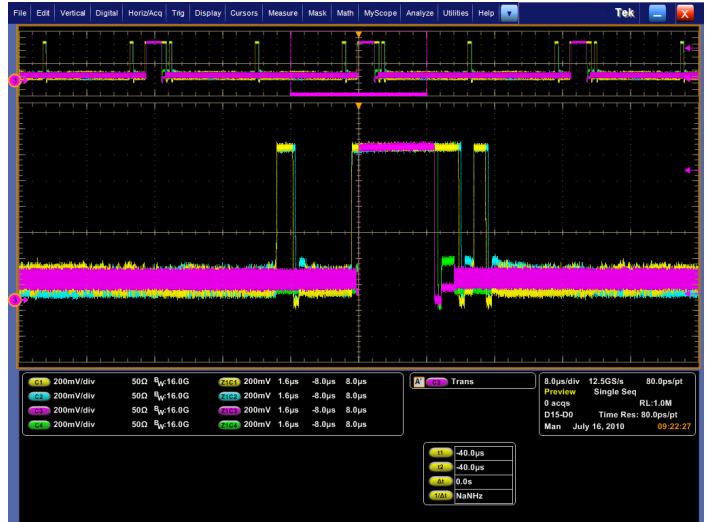
MIP® D-PHY Characterization and Analysis Solution (Option D-PHY) – Verify to the D-PHY specification by rapidly characterizing and discovering sources of jitter and signal integrity concerns using the fully flexible and customizable test setup. Using DPOJET, Option D-PHY enables transmitter high-speed data-clock timing measurements, along with a full range of electrical characteristics in high-speed or low-power modes.
