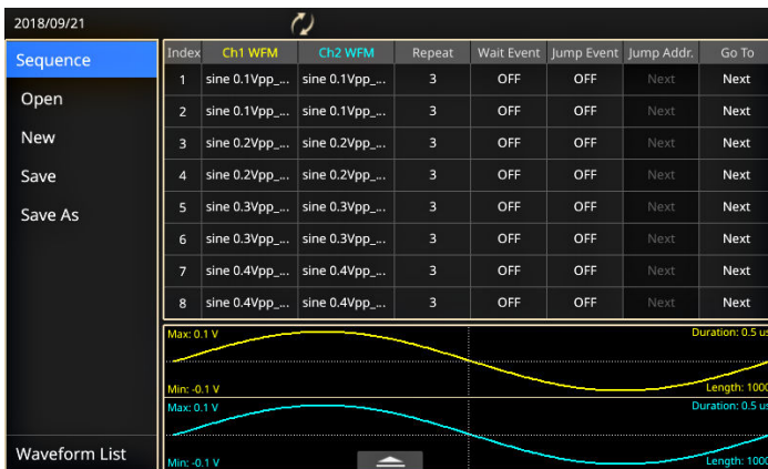
Figure 2: Advanced mode lets you build complex waveform sequences with flexible step controls
