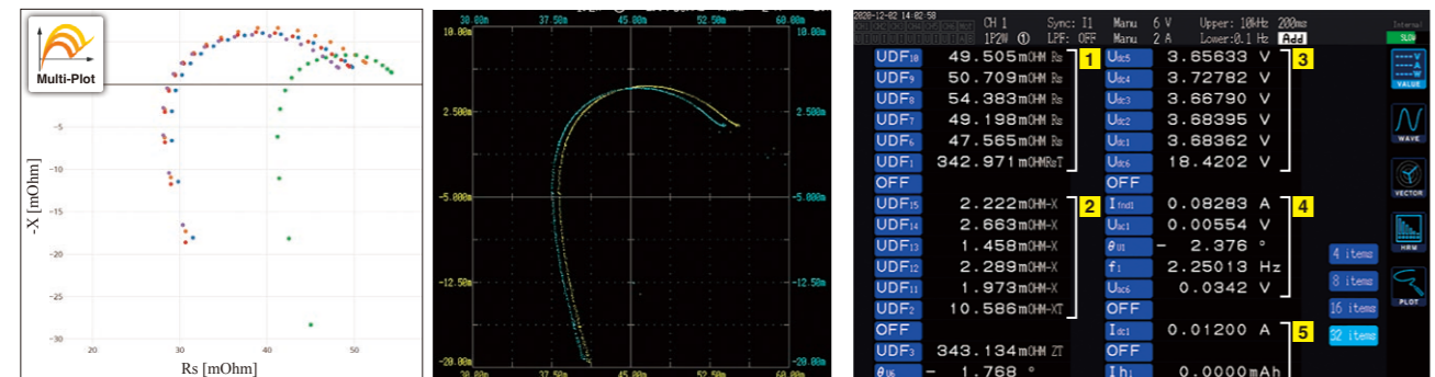
Left: Drawing Nyquist or Cole-Cole plots by the "Multi-plot" application. Right: Drawing Nyquist or Cole-Cole plots by the ALDAS-F. (Plots can be displayed for up to two channels.)
