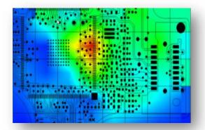
EMC and signal integrity are major concerns in the design of ultra-high speed (>2 GHz) PCBs. EMScanner enables the design engineers to diagnose EMC/EMI problems between 150 kHz and 8 GHz.
