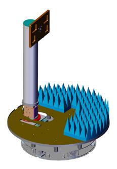
ETS-Lindgren's Model 2120CR Heavy Duty Multi-Axis Positioning System (MAPS) is designed to provide smooth rotation of a test object in both theta and phi axes. Typically the model 2120CR is used in systems that measure spherical antenna patterns and total effective radiated power of a wireless device, with MAPS units currently in operation at several CATL labs.
