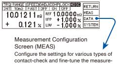
configure the settings for various types of contact-check and fine-tune the measurement timing.
