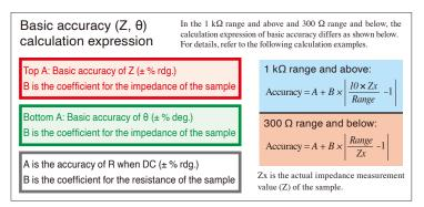
The measurement accuracy is calculated based on the following equation. Measurement accuracy = Basic accuracy  $\times C \times D \times E \times F \times G$
