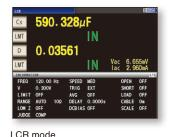
Cs and D display screen (120 Hz measurement)
