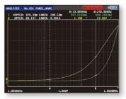
Frequency sweep measurement Z-θ measurement screen
