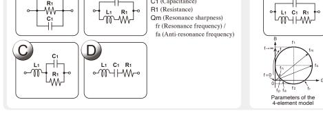
L1 (Inductance) C1 (Capacitance) R1 (Resistance) C0 (Parallel capacitance) Qm (Resonance sharpness or mechanical quality coefficient)
