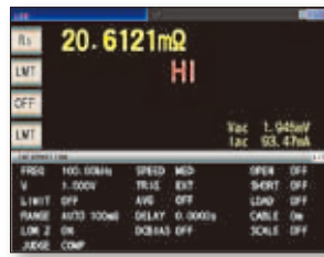
LCR mode Rs display screen (100 kHz measurement)
