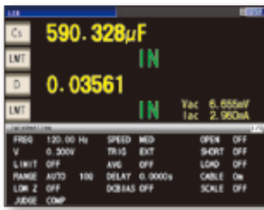
LCR mode Cs and D display screen (120 Hz measurement)
