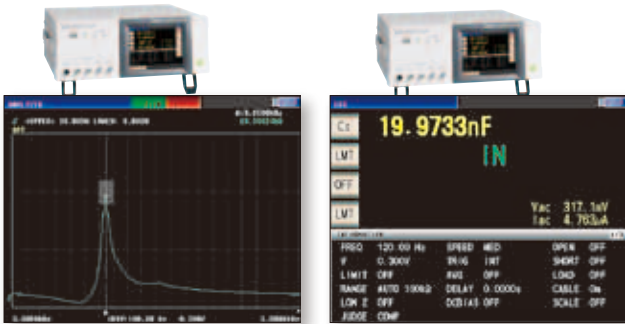
Frequency sweep measurement Z peak comparator screen
