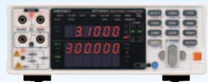
**Voltage measurement ranges:** 6V/60V/300V (BT3563)
