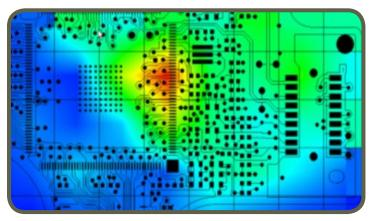
EMC and signal integrity are major concerns in the design of ultra-high speed (>2 GHz) PCBs. EHX enables the design engineers to diagnose EMC/EMI problems between 150 kHz and 8 GHz.
