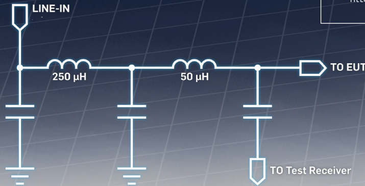
L3-64 equivalent circuit
