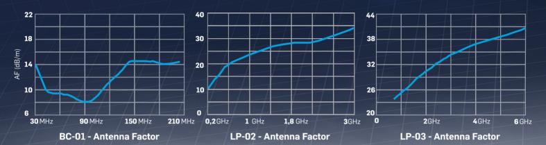
AS-03 antenna set 30 MHz to 6 GHz with individual calibration reports. AS-03/TC antenna set 30 MHz to 6 GHz with typical calibration reports. Includes: BC-01 biconical antenna, LP-02 log-periodic antenna, LP-03 log-periodic antenna, TR01 wooden column tripod, antenna mounting adapter to change polarization, 5 meter/6 GHz/N(m)-N(m) RF cable, N(f)-N(f) adapter, soft carrying case, user's manual, calibration reports\*
