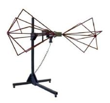
ETS-Lindgren's Model 3158 Biconical Antenna is a high power biconical designed for high level immunity. The Antenna can generate 100V/m over a ferrite covered ground at 2m distance per the ISO 11451-2 standard. The 3158 is a rugged version of the successful 3109 design. The 3158 has larger elements which reduce the VSWR at low frequencies. The rugged construction increases the power handling to 5 kW. It is a great antenna for generating higher fields in the 20 MHz to 120 MHz frequency band.
