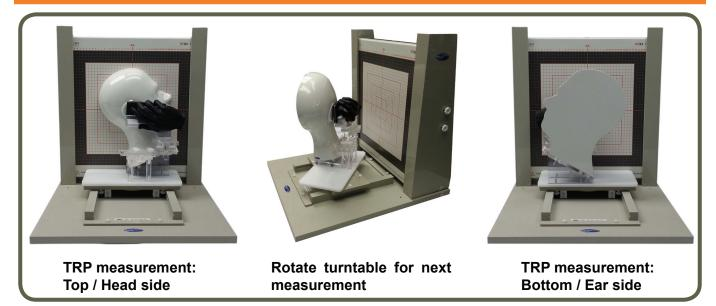
TRP measurement: Rotate turntable for next TRP measurement: 'Head' side measurement 'Ear' side
