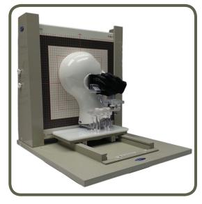
Mobile devices can be placed repeatedly against the RFX2 and provide TRP measurements in seconds. To obtain
