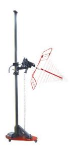
ETS-Lindgren's Model 2171B Antenna Tower meets ANSI C63.4 requirements for measurements above 1 GHz by keeping the antenna aimed at the EUT during the antenna's ascent/descent along the antenna mast. This is especially useful when high gain directional antennas like horn antennas are used. This antenna tower is also designed with a reduced size base for better maneuverability in smaller chambers.
