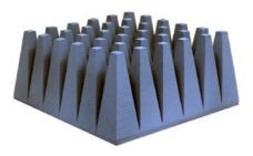
ETS-Lindgren's FerroSorb FS-300 EMC Absorber is part of the FS Family of hybrid (ferrite tile and carbon loaded material) absorbers from ETS-Lindgren. The FAA-300 loaded foam portion is designed to match the impedance of ETS-Lindgren's FT-1500 Ferrite Tile panels. When combined, these two absorber technologies become the FS-300 absorber system.
