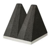
ETS-Lindgren's DuraSorb DSH-600H Absorber is the latest evolution of ETS-Lindgren's low profile, hybrid anechoic absorber technology. It combines the advantages of the proven FerroSorb performance with the physical properties of the PS Series absorbers. DuraSorb is constructed using substrates with rigid, closed cell foams, which are loaded volumetrically and uniformly throughout the absorbers. DSH-600H is ideal for 3 m range and 5 m range chambers.
