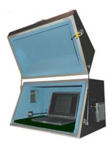
ETS-Lindgren's Model 5225-2 Benchtop Test System has been developed for testing medium-sized wireless devices, such as laptop computers. The unit is constructed of durable welded aluminum and features a large clamshell lid with pneumatic springs and dual locking latches. Flat RF absorber lines the interior and greatly reduces resonant behavior in the cell.
