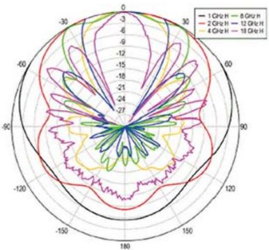
Model 3164-11 Open Boundary Quad-Ridged Horn Typical Radiation Patterns Cross Port Coupling
