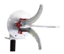
ETS-Lindgren's Model 3164-11 Open Boundary Quad-ridged Horn is the latest in a series of quad-ridged horns from ETS-Lindgren. The "open boundary" design with its absence of side plates makes this antenna unique in both appearance and performance. Numerically modeled, the Model 3164-11 is a super open boundary quad-ridged horn where the feed cavity is not enclosed. This gives wider frequency range and reduces the weight of the horn.
