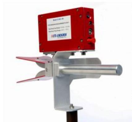
ETS-Lindgren's Model 3116C-PA is a special version of our popular Model 3116C Double-Ridged Waveguide Horn Antenna, fitted with a pre-amplifier package and calibrated as a single unit. By doing this, any possible mismatches between antenna and pre-amplifier are taken into account in the antenna factor (AF), which is provided with this unit.
