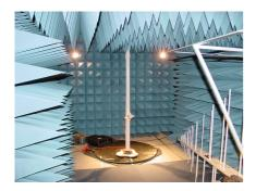
ETS-Lindgren's SpaceSaver<sup>TM</sup> PC is a semi-anechoic chamber, designed to perform ANSI C63.4/CISPR 16-1-4 and IEC 61000-4-3 pre-compliant radiated immunity measurements. This chamber can also be used for ANSI C63.4 pre-compliant radiated emissions measurement pre-scans, with limited height scan. Frequency ranges for this chamber are 80 MHz to 40 GHz (radiated immunity) and 30 MHz to 40 GHz (radiated emission).
