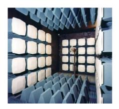
ETS-Lindgren's SpaceSaver™ FAR chambers are designed to perform IEC 61000-4-3 compliant radiated immunity measurements. Fully anechoic, these chambers can also be used for CISPR 16-1-4 pre-compliant radiated emissions measurement pre-scans, with fixed height. Frequency ranges for this chamber are 26 MHz to 40 GHz (radiated immunity) and 30 MHz to 40 GHz (radiated emission).
