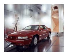
ETS-Lindgren's SMART<sup>TM</sup> (Statistical Mode Averaging Reverberation Test-Site) Chambers use the latest developments in proven reverberation technology and experienced chamber design and construction, to create a suitable electromagnetic environment (EME) for immunity, emissions and shielding effectiveness testing. Compared with other test methods, SMART chambers offer the advantages of lower cost, higher field-to-input power ratios, and the ability to accept large test systems.
