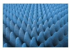
ETS-Lindgren's Convoluted Absorber is designed to provide good refectivity performance with low forward scattering characteristics at incident angles up to 60° from normal incidence at microwave and millimeter-wave frequency ranges.
