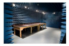
ETS-Lindgren's MIL-STD-461 chamber is designed for testing in accordance with Mil-Std 461E, Mil-Std 461F and Mil-Std-461G. The chamber's shell is constructed with Series 81™ modular cell-type shielding panels. Interior end walls, portions of the sidewalls and ceiling are lined in the manner required by MIL-STD-461, using EMC-24PCL absorber.
