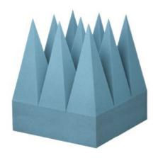
ETS-Lindgren's EMC-24PCL EMC Absorber is an ultra broadband microwave absorber which has been optimized for EMC applications. Its design is an evolution of traditional pyramidal polyurethane absorber and combines carefully balanced dielectric properties with a special geometry that is suited for low frequency operation.
