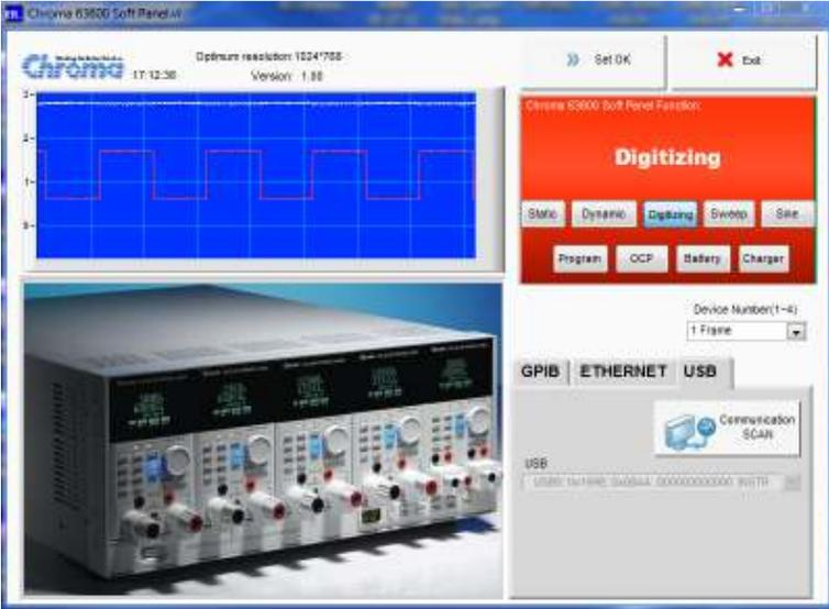
Figure 1 The 63600 Softpanel interface screen
