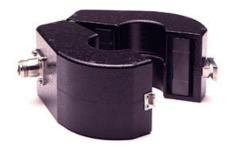
ETS-Lindgren's Model 94111-1 Current Probe is capable of making bulk current injection measurements up to 1 GHz. The 94111-1 is a RF sniffer probe for cable common mode current sources of radiated emissions and as measurement of cable common mode coupled currents during radiated susceptibility testing.
