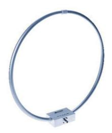
ETS-Lindgren's Model 6512 has a frequency range of 9 kHz - 30 MHz and is a passive loop antenna designed for both emissions and immunity tests. Every loop antenna can be individually calibrated in accordance with the IEEE-291 Section 2.3.1 methods, using NIST traceable equipment. By knowing the actual antenna factors and performance characteristics of an antenna instead of typical data, you can more accurately measure field strength in your tests.
