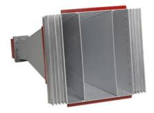
ETS-Lindgren's Model 3162-01 Field Generating Pyramidal High Gain Horn was specifically developed for the GMW 3097 and ES-XW7T-1A278-AC specifications for radar pulse testing. These tests require that the EUT be exposed to a pulsed peak field level of 600 V/m at a distance of 100 cm (3.28 ft) from the front of the horn.
