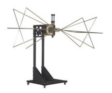
ETS-Lindgren's Model 3159C Biconical Antenna is a broadband, linearly-polarized biconical antenna. The 3159 Biconical Antenna exhibits a wide beamwidth and is specially designed to handle up to 10 kW input power for generating high electric field strength over a large uniform area.
