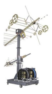
ETS-Lindgren's Model 3152 is a dual array of LPDA antennas based on the successful ETS-Lindgren Model 3148B. With a frequency range of 200 MHz to 1 GHz, this antenna's array arrangement provides an additional gain improvement of 3 dB across the range, and a convenient space-saving design with the use of top hat-loaded, low-frequency elements. (Product photo shows Model 3152 mounted with Foreshortened Log Periodic Array mounted on a custom ETS-Lindgren positioning mast)
