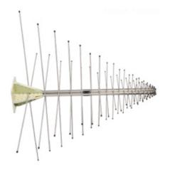
ETS-Lindgren's Model 3145BDP Dual-Polarized Log-Periodic Array is a dual linearly polarized, broadband antenna designed to operate over the frequency range of 100 MHz to 1.1 GHz. The choice of scaling factors, the various diameters of each element, and the center-to-center spacing of the booms result in excellent VSWR characteristics throughout the operating frequency range.
