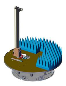
ETS-Lindgren's Model 2115CR Medium Duty Multi-Axis Positioner is designed to provide smooth rotation of a test object in both theta and phi axes. Typically the model 2115CR is used in systems that measure spherical antenna patterns and total effective radiated power of wireless devices, with MAPS units currently in operation at several CATL labs. Options include the SAM Phantom (head) and ETS-Lindgren's Positioning Controller with GPIB and EMQuest<sup>™</sup> Software.
