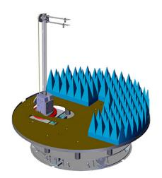
ETS-Lindgren's Model 2110CR Light Duty Multi-Axis Positioning System is designed to perform measurements of spherical antenna patterns, plus total and effective isotropic radiated power of wireless hand-held devices.
