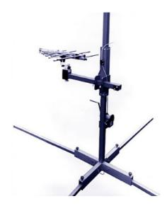
ETS-Lindgren's Model 1052 Portable Antenna Tower is useful for quick measurements, pre-scans, and anywhere a portable tower is needed. The model 1052 has two fiberglass mast sections, a hand winch, and four extending aluminum legs that are easily assembled/disassembled for ease of transportation.
