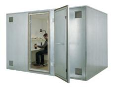
ETS-Lindgren's Series 101 RF shielded construction system meets and substantially exceeds all RF shielding requirements. The system consists of modular, hot galvanized rigid steel structural panels and can be dismantled and reinstalled, enlarged or modified due to the panel system (only the gasket and the fasteners have to be replaced). No special tools nor welding are necessary during the installation and no maintenance is necessary after installation.
