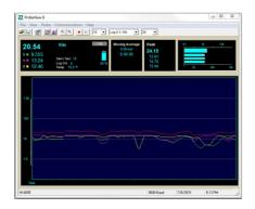
ETS-Lindgren's ProbeView™ Software is designed for use with the HI-4413P or HI-44USB fiber converters. ProbeView™ enables user-selectable viewing options (numeric or graphical), selectable logging, simultaneous display of peakhold and current field strength data, and graphical representations of field strength versus time.
